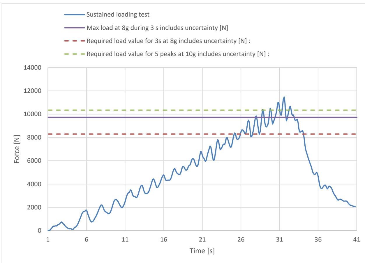
**Sustained loading test results <sup>(3)</sup>**
